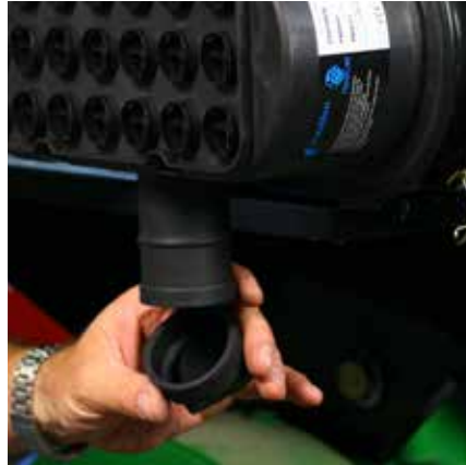
The Donaldson Vacuator™ Valve can be found on the majority of Donaldson air cleaners.
